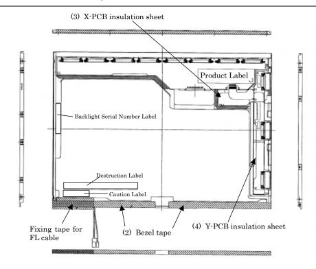
Figure 4-51 Replacing TMD fluorescent lamp (WXGA) (1)
